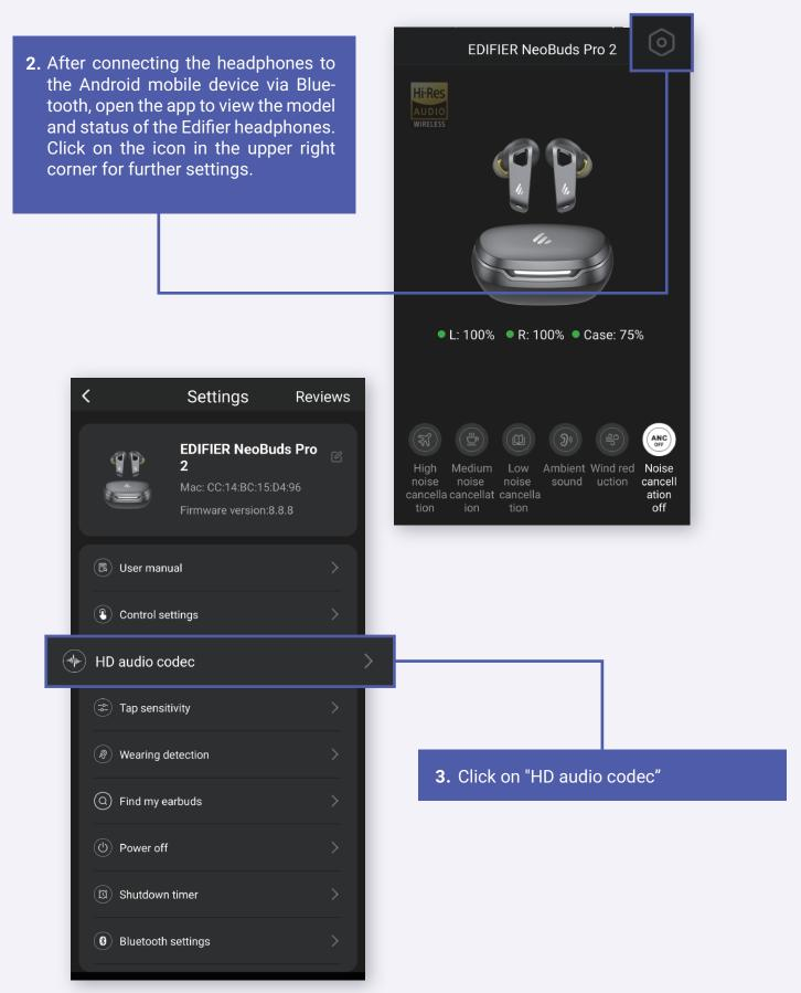
HD audio codec Save 4. Enable the "192kHZ Sampling Rate" Enable the LDAC or LHDC HD audio codec feature for LHDC, then click on the "Save" button in the upper left corner to bitstream of LDAC or LHDC, compatibility differences complete the setup. LHDC audio codec **LDAC** Sampling rate of 96kHz  $\bigcirc$ Sampling rate of 44.1kHz/48kHz Disable LDAC  $\bigcirc$ **LHDC** Sampling rate of 192kHz 0
